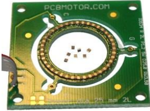
Figure 6 – Stator with piezo components in center
