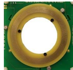
Figure 13 – 40mm hollow center rotor.
