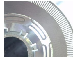
Figure 12 – Close-up of hollow shaft rotor.
