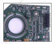
Single motor, one-layer design (Ø30 mm stator) with an integrated driver based on customer specifications.
