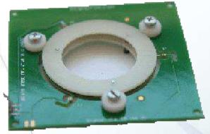
Hollow 60 mm rotor construction with 3 rollers.
