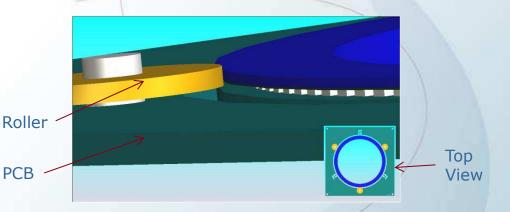
3-point roller support principle for radial alignment.
