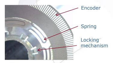
12 mm 'free center' using a rotor disc for Ø30 mm stator with spring & sensor markings.
