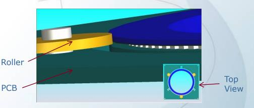
3-point roller support principle for radial alignment.
