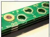
5 motor, two-layer design (Ø25 mm), one central driver in a *sandwhich* construction. Upper & lower decks contain the motors, with the driver placed on the center board.
