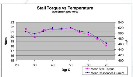
An operating temperature range of -10 to 85 C has been tested and confirmed in some applications.
