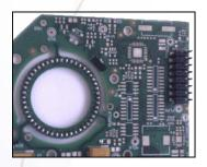
Single motor, one-layer design (Ø30 mm stator) with an integrated driver based on customer specifications.
