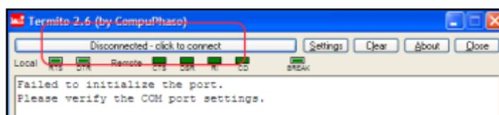
4. Go back to *Settings, Ports* and click the down arrow ‘↓’ to see the number of the port that was assigned to the High Resolution Twin Motor Kit. Select the corresponding port and click *OK*. Termite will now display “Termite is initialized and ready.”
